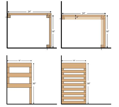
**Top View:** : Shows screw location and sizes. Second picture shows an optional cap piece with 45° Miter.
