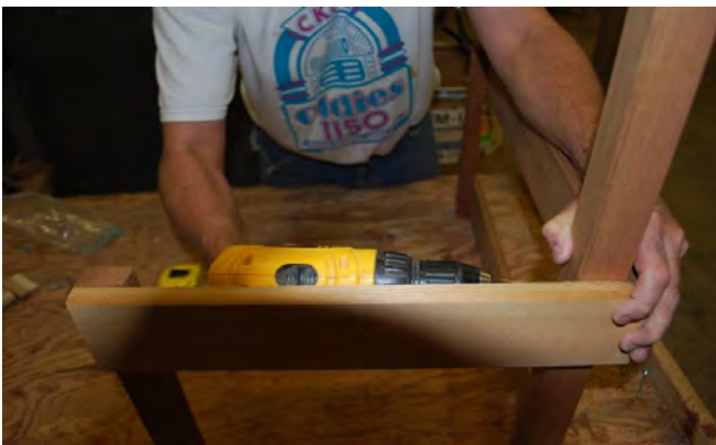
130. Stand up 1x4 and 2x2 leg assembly. Line up 1x4's and screw together.
