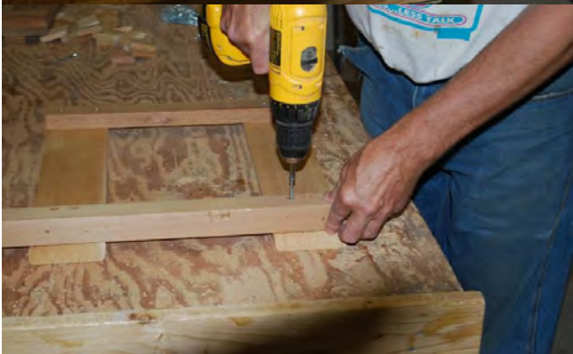
127. Determine which way the heater guard is to be mounted then screw 2x2 heater guard leg to 1x4 horizontal.
