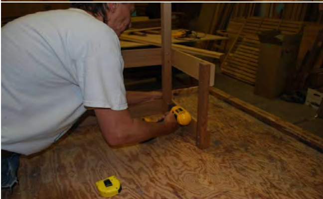
131. Line up remaining 1x4's and screw together.
