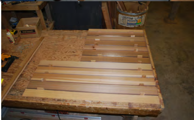
152. Making the floor. The duckoatd floor only covers the walking area in front of the benches. Measure floor area after benches and heater guard in place. Cut floor boards to measurement. Layout floor with good face down and 1/2" space between boards. Since good face is down make sure that when you flip to the good face up it will be the proper layout.
