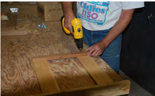
126. Assembling 2 sided heater guard. Screw 15" verticals to horizontal 1x4.
